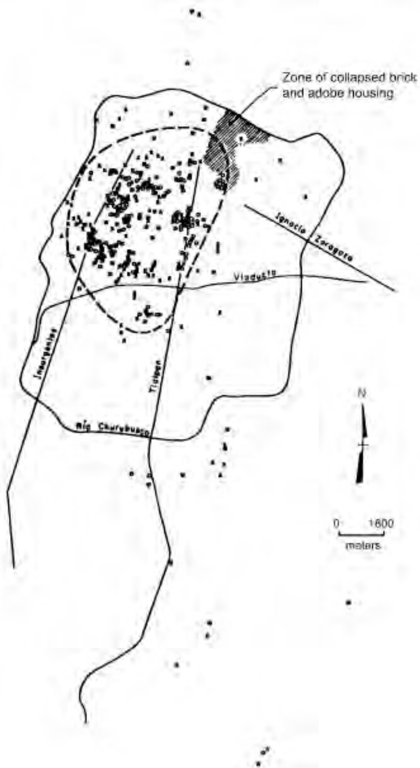
FIGURE 30.30 Locations of building damage at Old Lake Bed in Mexico City. (Courtesy of EERI [2].)
