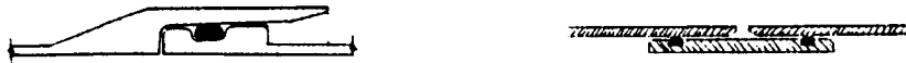
FIGURE 25.2: Bell-and-spigot and coupling joints for fiberglass pipe. (From American Society for Testing and Materials. 1991. D3517. Standard Specification for "Fiberglass" Glass-Fiber-Reinforced Thermosetting-Resin Pressure Pipe . With permission.)
