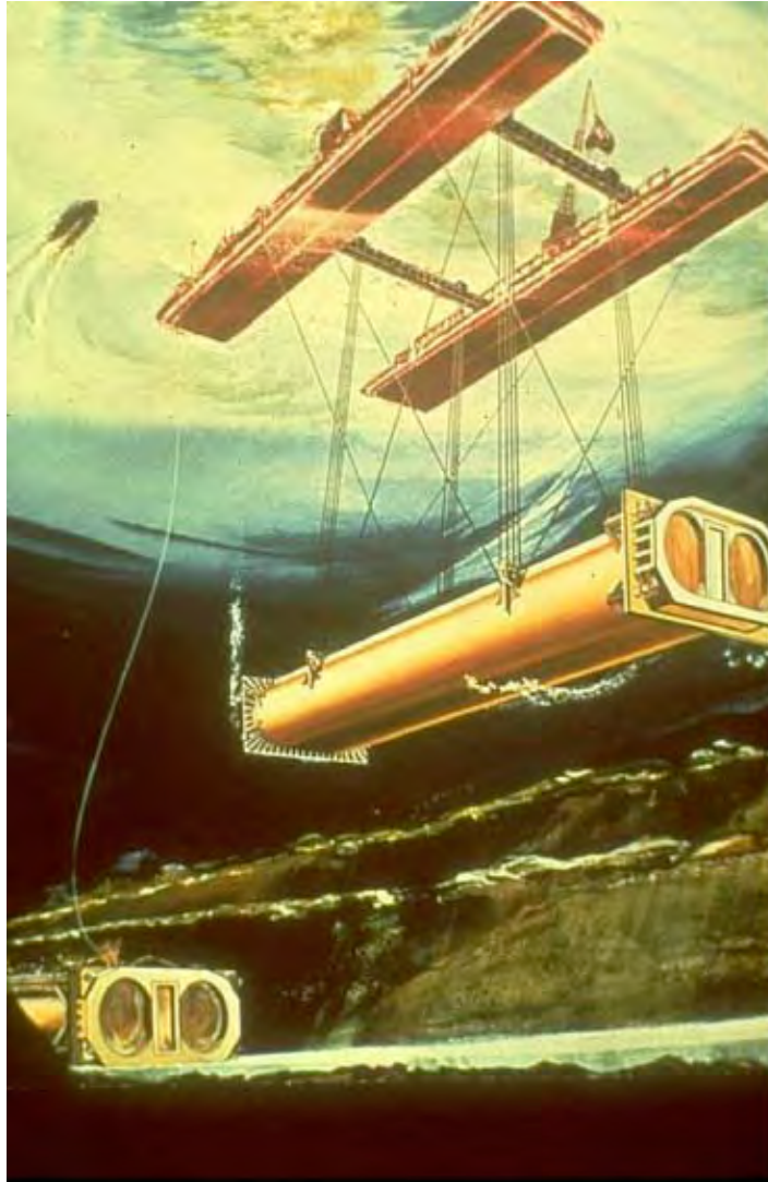
FIGURE 15B.1 Lowering an immersed tunnel element into the excavated trench. (© Parsons Brinckerhoff, Inc., 1967. With permission.)
