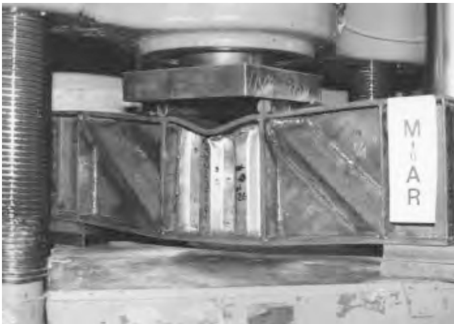
FIGURE 19.15: Bending failure of a beam with corrugate web.
