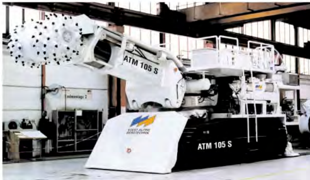
FIGURE 15B.14 Roadheader with double rotating cutterhead. (©2000 Sandvik. With permission.)
